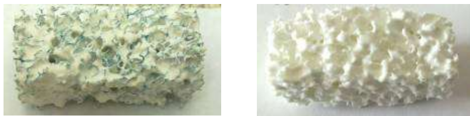
Fig. 1. Polyurethane foam coated with ceramic slurry and dried at RT (left) and sintered ceramic foam (right)
