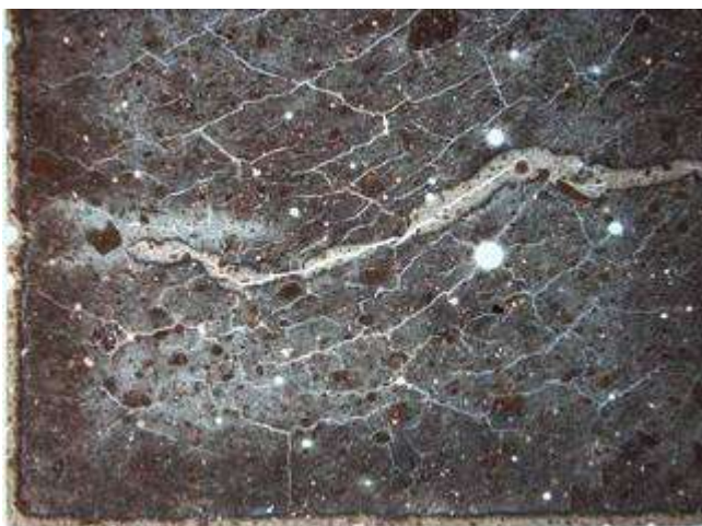
Fig. 1. Optical microscopy in transmitted light for 28-day paste cured at 100% relative humidity. High concentration of cracks is visible in the inner zone.
